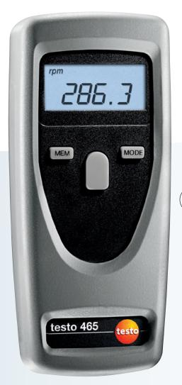
With the testo 465, you can measure rpm easily without contact using only one hand. The measuring instrument is thus suitable for measurements on rotating parts such as ventilators and shafts. Simply attach a reflective marker (optional) to the measurement object, point the visible red beam of light at the reflective marker, and measure. The
